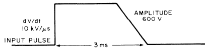
Fig.16 - Waveforms showing response of a 100-millihenry solenoid control circuit to a fast-rising transient.
